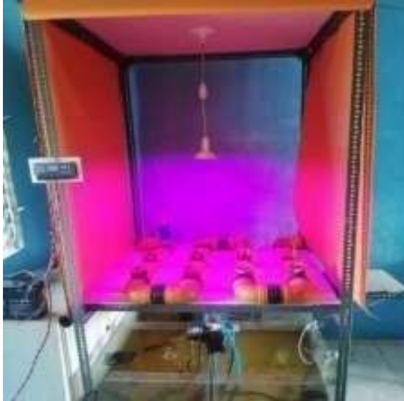
Figure 3 shows the outcome design of created aquaponics system – its embedded sensors, and grow light.
