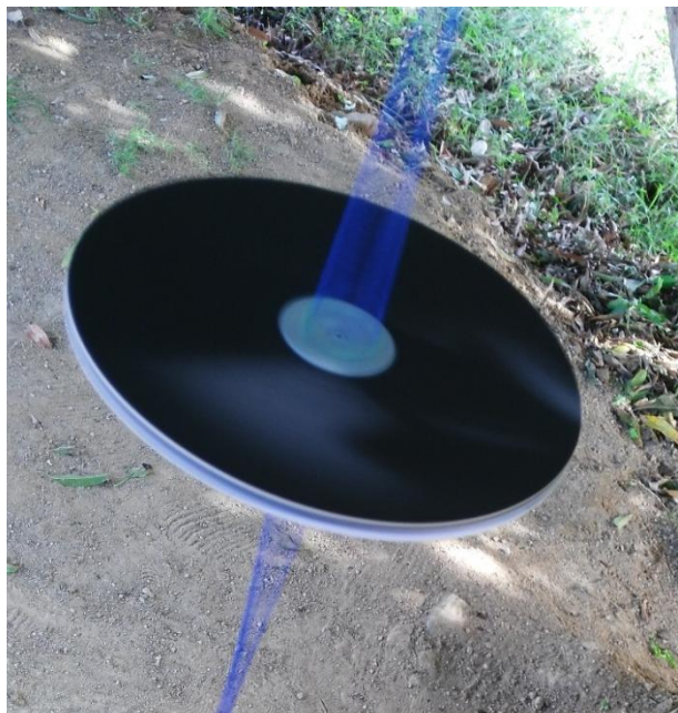
Figure 1. The spinning modified paperfuge
